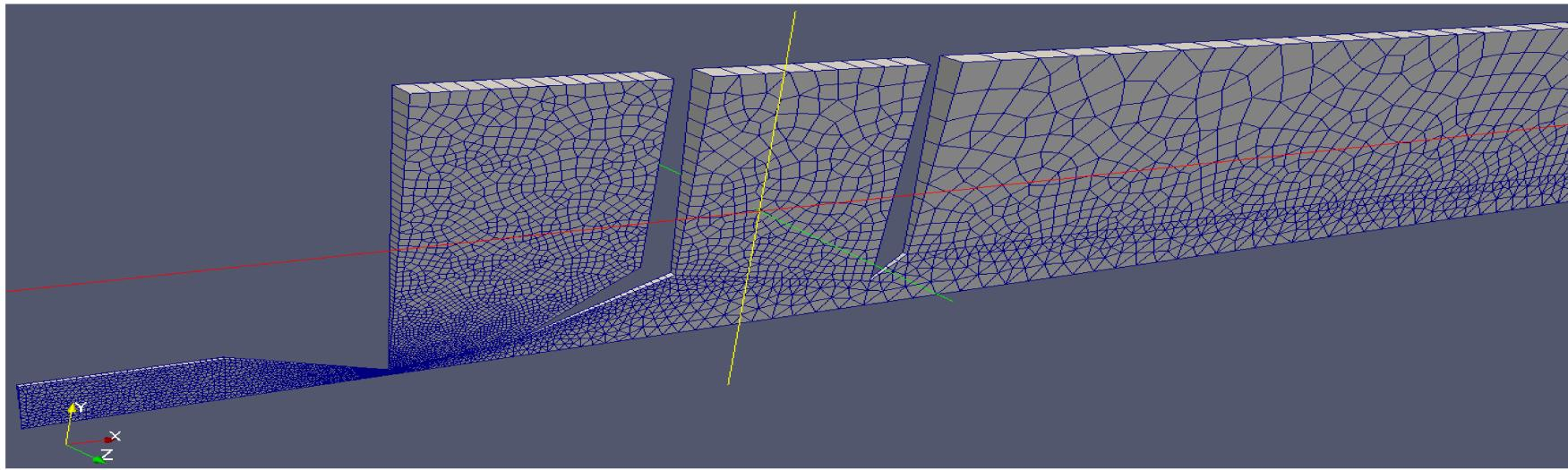
Mix of triangles and quadrilaterals, cell size should be of the order of the mean free path length of the particles
