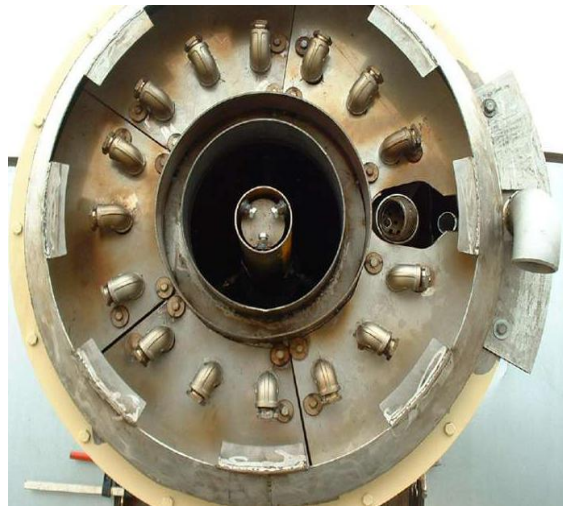
The burner for industrial means with 10 megawatt output power.
