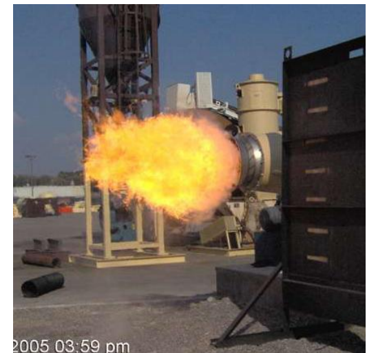
The burner for industrial means with 10 megawatt output power.
