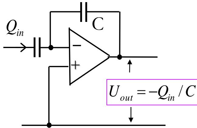
The output voltage is changed, until the charge via **C** compensates  $Q_{in}$  from the input
