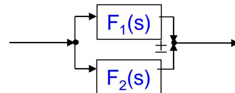
$$T(s) = F_1(s) \pm F_2(s) \quad (\text{Linearity})$$
