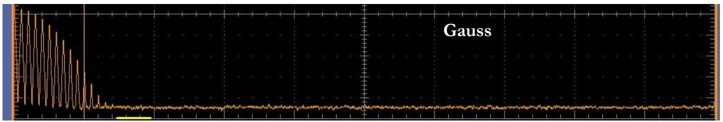
Semi-Gaussian pulse shaping has the fewest harmonics and allows to amplify these pulses with the comparatively smallest bandwidth.
