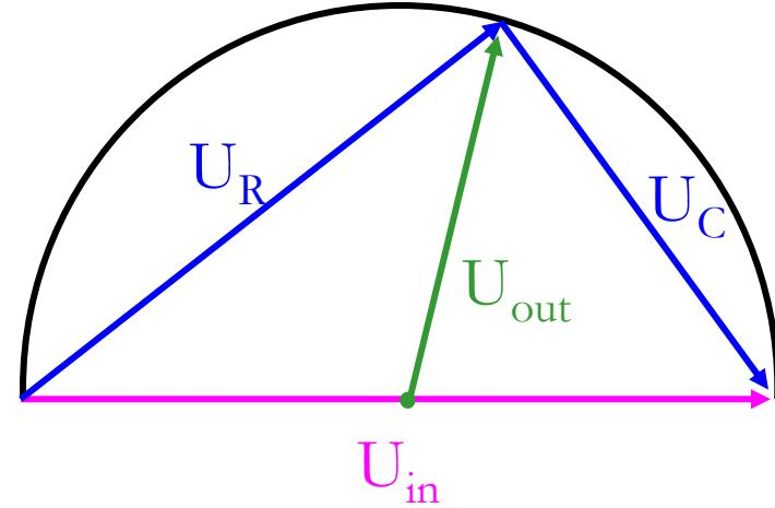
$$U_{\text{out}} = U_{R_1} - U_C = \frac{1}{2} U_{\text{in}} - \frac{R_C}{R + R_C} U_{\text{in}}$$
