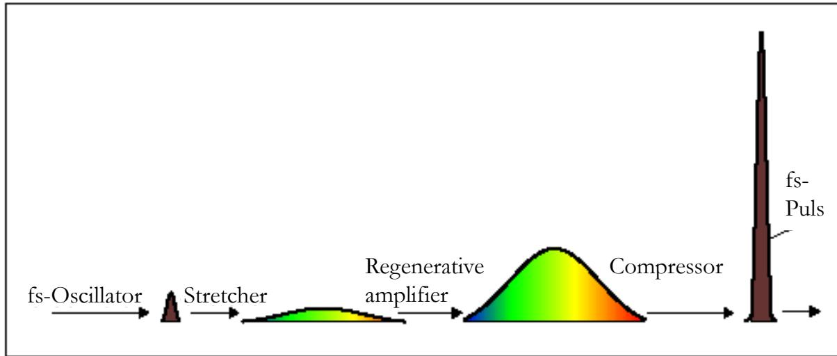
Principle of the CPA : High peak intensities within the amplifier optics are avoided by timewise and spatial dilatation of the pulses.
