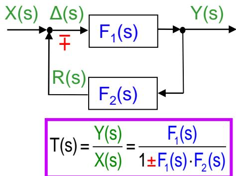
$$\left. \begin{aligned} Y(s) &= F_1(s) \cdot \Delta(s) \\ \Delta(s) &= X(s) - R(s) \\ R(s) &= F_2(s) \cdot Y(s) \end{aligned} \right\} \rightarrow Y(s) = F_1(s) \cdot \{X(s) - (F_2(s) \cdot Y(s))\}$$
