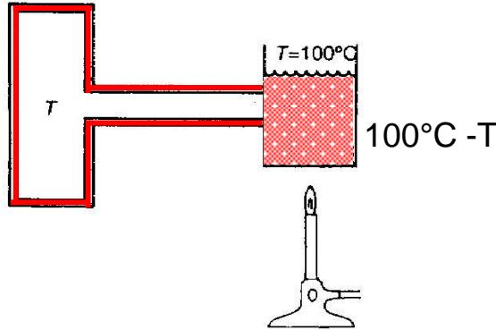
The temperature of a piece of metal approaches exponentially  $100^\circ\text{C}$ .
