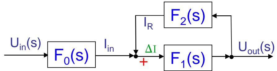
$$T(s) = F_0(s) \cdot \frac{F_1(s)}{1 - F_1(s) \cdot F_2(s)} \xrightarrow{F_1(s) \rightarrow \infty} \frac{F_0(s)}{-F_2(s)} = -\frac{Z_2}{Z_1}$$
