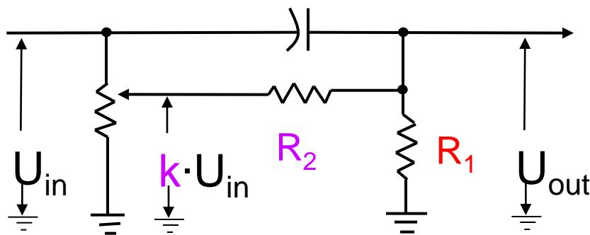
$$R_P = R_1 \parallel R_2 = \frac{R_1 \cdot R_2}{R_1 + R_2}$$
