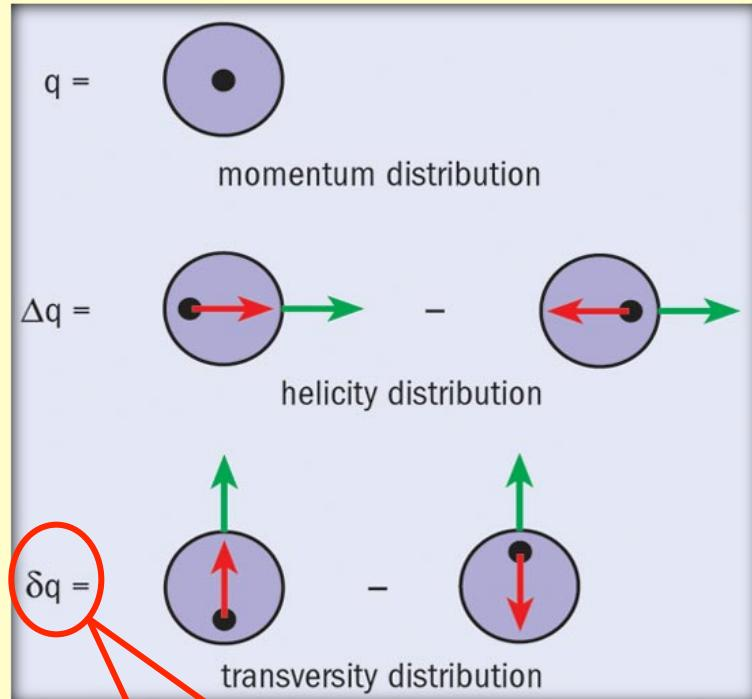
$$A_{TT} \equiv \frac{d\sigma^{\uparrow\uparrow} - d\sigma^{\uparrow\downarrow}}{d\sigma^{\uparrow\uparrow} + d\sigma^{\uparrow\downarrow}} = \hat{a}_{TT} \frac{\sum_q e_q^2 h_1^q(x_1, M^2) \bar{h}_1^q(x_2, M^2)}{\sum_q e_q^2 q(x_1, M^2) \bar{q}(x_2, M^2)}$$
