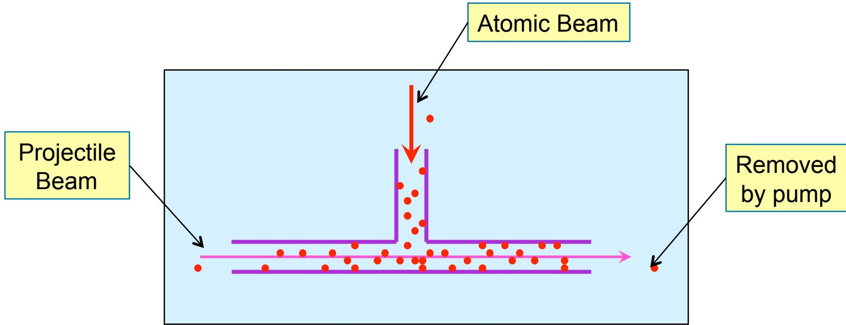
After each wall collisions, atoms can intercept beam again.
