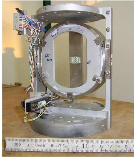
Fig. 4.9. : Crystal support with crystal and aluminum aperture of 60 mm width. On the bottom left side the servomotor with linear potentiometer for tilting of the mirror is shown.
