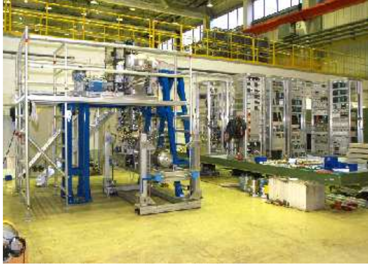
Figure 9: Polarised Internal Target installation at the off-beam position. The blue pillars on the left that support the bridge on which the ABS is mounted, exactly mimic the D1 and D2 magnets of ANKE.
