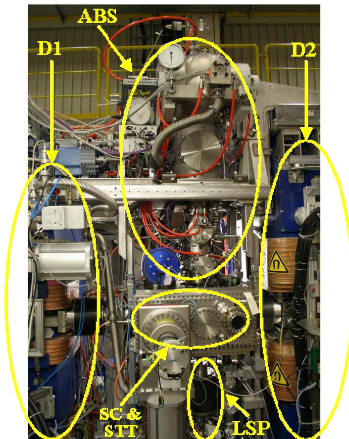
**Fig. 1.** Photo of ANKE with the Polarized Internal Target (PIT) installed between the beam bending magnet D1 and the spectrometer dipole magnet D2. The main components of the PIT system are: Atomic Beam Source (ABS), Lamb-shift Polarimeter (LSP), and the target chamber supporting the Storage Cell (SC) together with Silicon Tracking Telescope (STT) system. The COSY beam enters the setup from the left.
