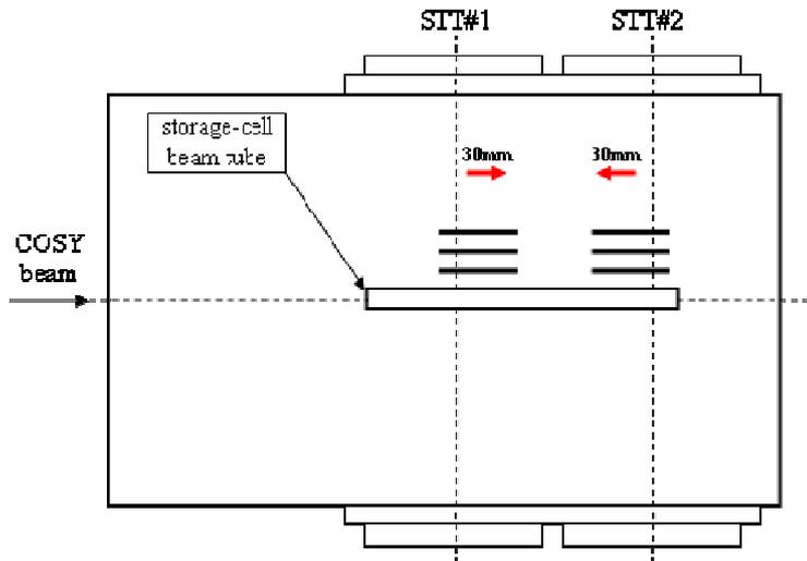
Fig. 7. Position of the STT at the ANKE target chamber.
