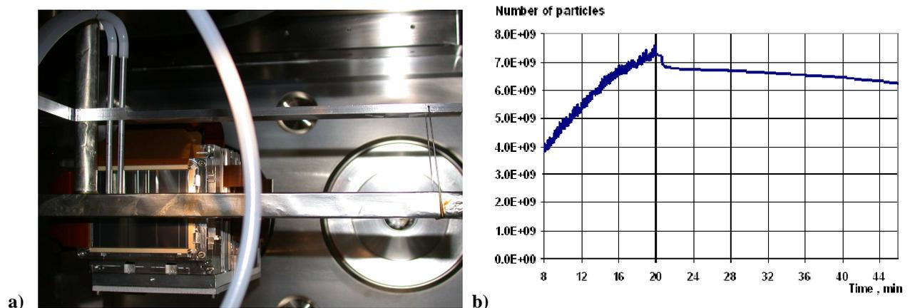
**Fig. 2. a)** The storage cell installed in the target chamber together with the Silicon Tracking Telescope (STT) system behind the cell. Two Teflon tubes, coming from the top, are used for the unpolarized gas feeding. **b)** The number of stored protons in the ring during stacking (120 stacks) through the storage cell followed by 10 s of electron cooling and accelerating to the flat top energy.
