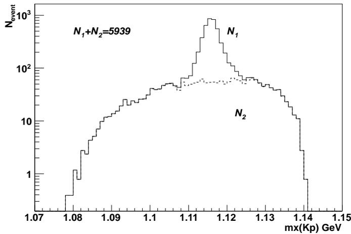
Figure 1: Simulation of the expected  $K^+p$  missing-mass spectrum for the  $pp \rightarrow K^+p\Lambda$  reaction at 2.425 GeV/c for the sum of all polarisation states after ten weeks of beam time. The peak in the distribution at the  $\Lambda$  mass corresponds to the detection of the direct proton from the reaction ( $N_1$ ), while the smooth distribution underneath arises from the  $\Lambda$  decay proton ( $N_2$ ) detected in coincidence with the  $K^+$  in the positive detector.
