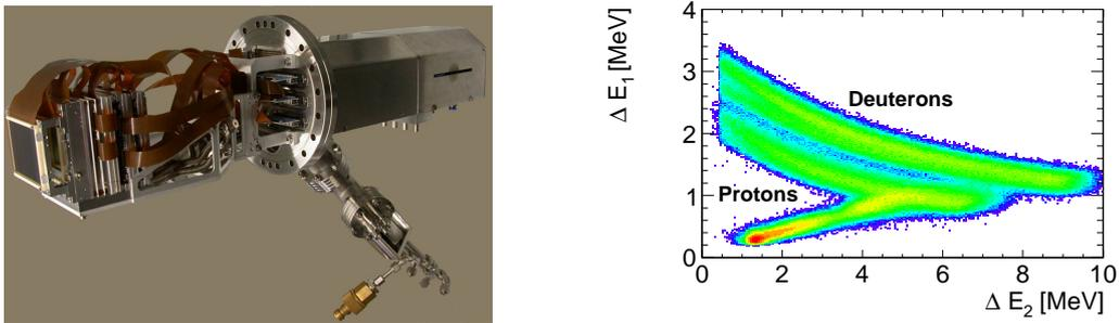
Figure 3: Left: Silicon Tracking Telescope consisting of three detector layers of different thickness. Right: Energy loss correlation for the first and second layers of the STT showing the separation of protons from deuterons in a logarithmic  $z$ -scale.
