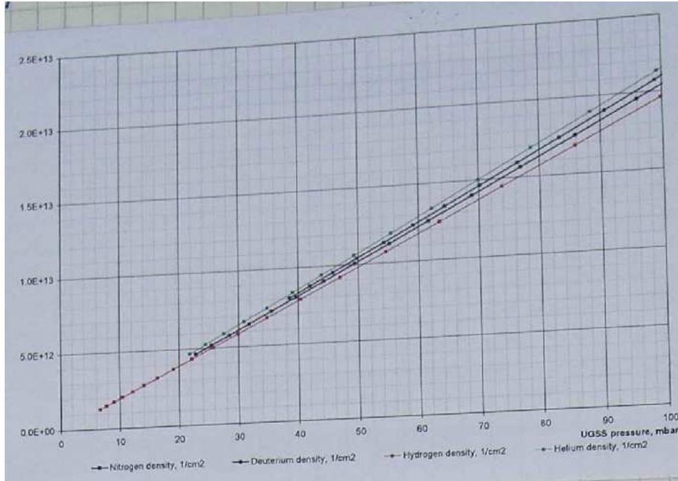
Figure 13: Calibration curve: Target density in particles /  $\text{cm}^2$  versus pressure in the unpolarized gas supply system (UGSS).
