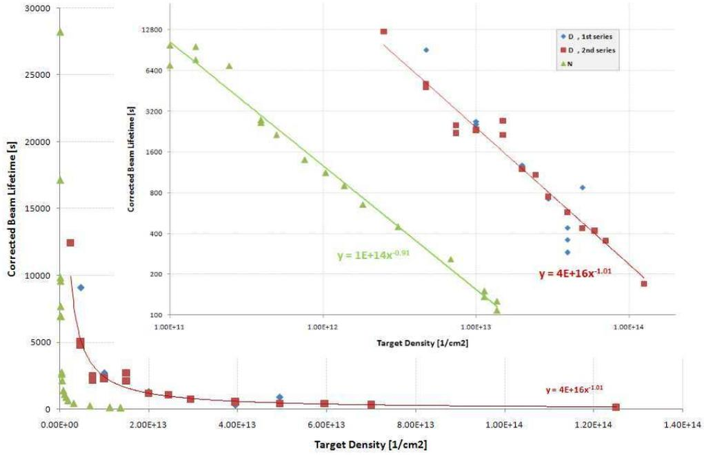
Figure 27: Beam lifetime dependence of the target density and a fit curve with the exponent as a fit variable for deuterium and nitrogen targets. The densities given here are atomic ones.
