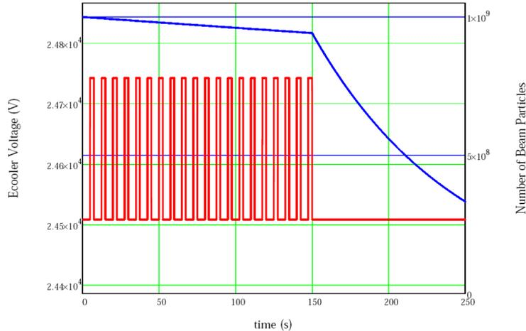
Figure 6: Cycle setup with alternating periods of detuned (2.5 s) and nominal (5 s) voltages of the electron cooler.
