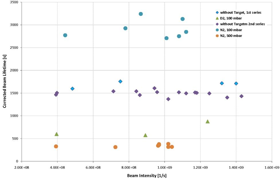
Figure 30: The lifetime dependence on the beam intensity for different gases and target densities .
