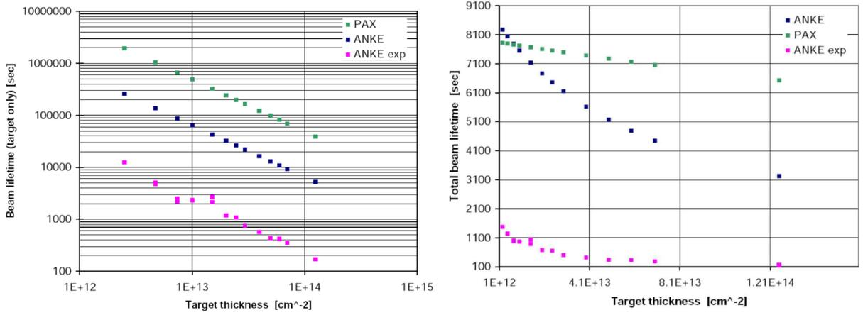
Figure 1: Measured beam lifetimes with (left panel) and without (right) background subtraction at the ANKE target location (magenta) using a  $D_2$  storage cell target at  $T_p = 45$  MeV. The other two sets are the result of a calculation of the expected beam lifetimes for ANKE (blue) and the location at TP1, where we anticipate to install the instruments for the spin-filtering studies (green PAX).
