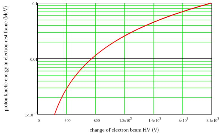
Figure 4: Proton energy in the electron rest frame as function of the necessary voltage change in the electron cooler.
