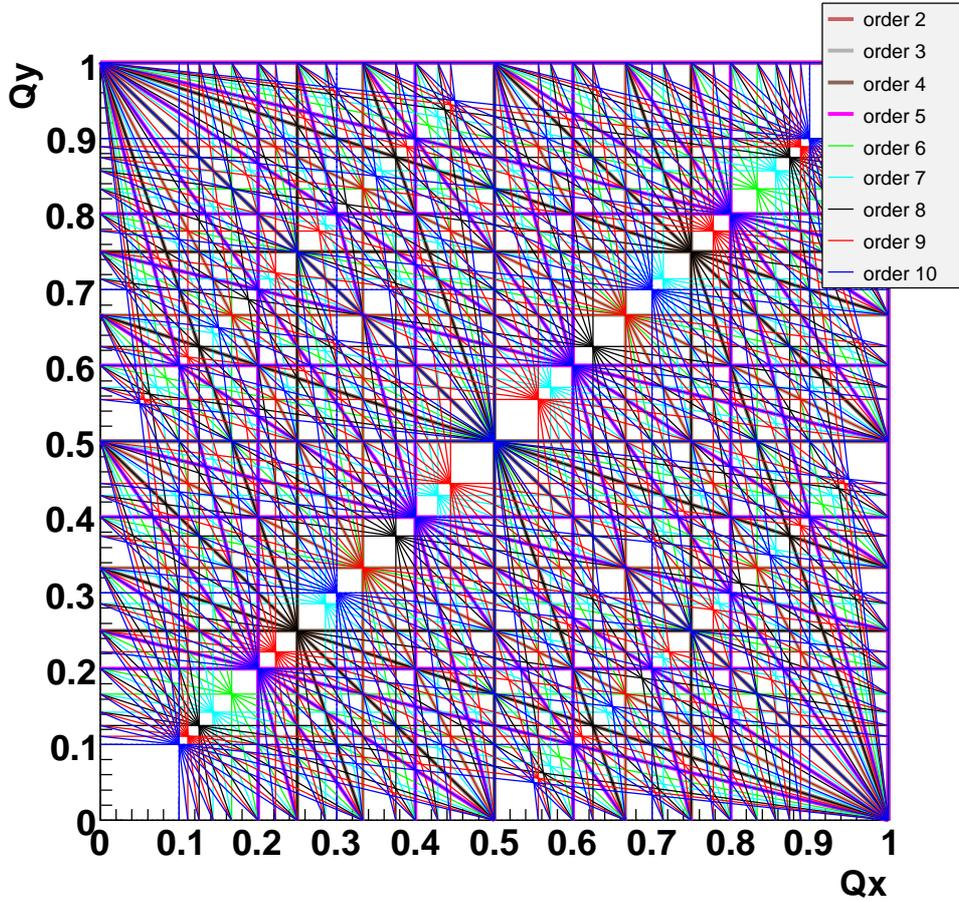
Figure 20: Fractional machine resonances up to the 10<sup>th</sup> order.
