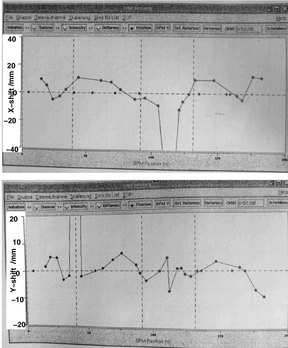
Figure 15: Beam orbit with electron-cooler magnets switched on.
