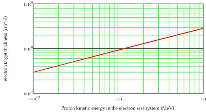
Figure 2: Calculated electron target thickness in the cooler for the proton energies of interest ( $I_e=240$  mA,  $l_{\text{Cooler}} = 2$  m, cross section of electron beam =  $5 \text{ cm}^2$ ).
