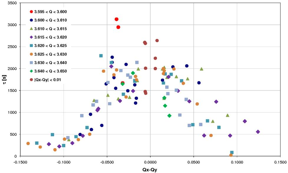
Figure 22: Beam lifetime as a function of tune difference. Each colour denotes a constant tune  $Q = \sqrt{\frac{Q_x^2 + Q_y^2}{2}}$ .
