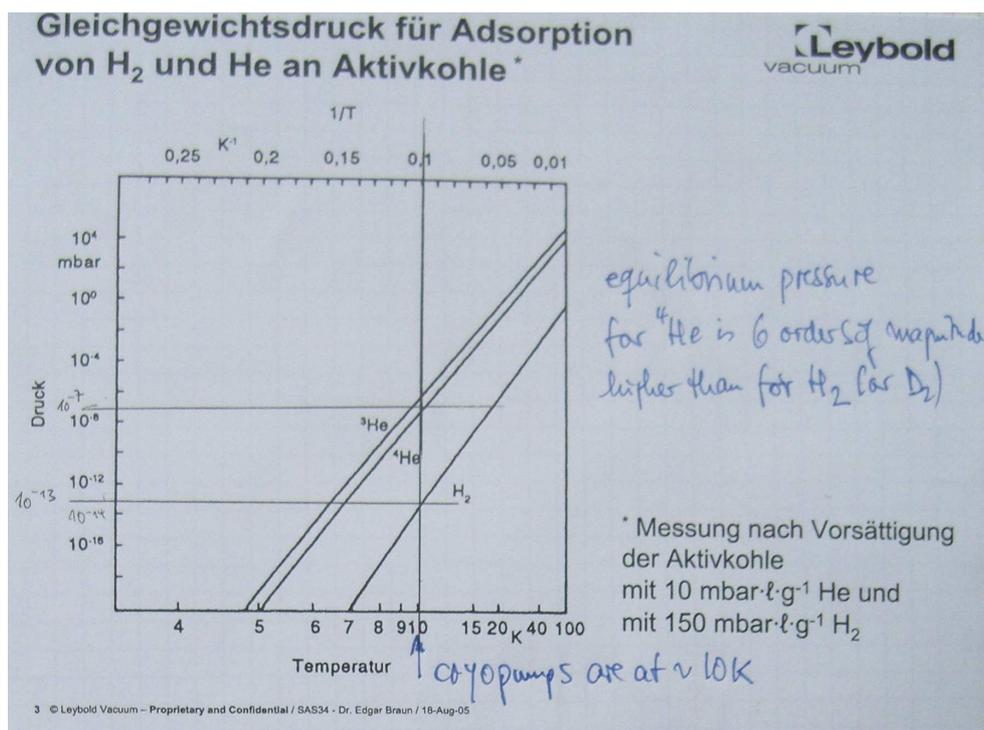
Figure 29: Equilibrium pressure for absorption of  $H_2$  and He with active coal.
