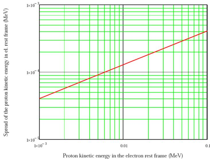
Figure 5: Absolute spread of the proton beam energy in the electron rest frame assuming a relative beam momentum spread of  $10^{-4}$  as function of the proton kinetic energy in the electron rest frame.
