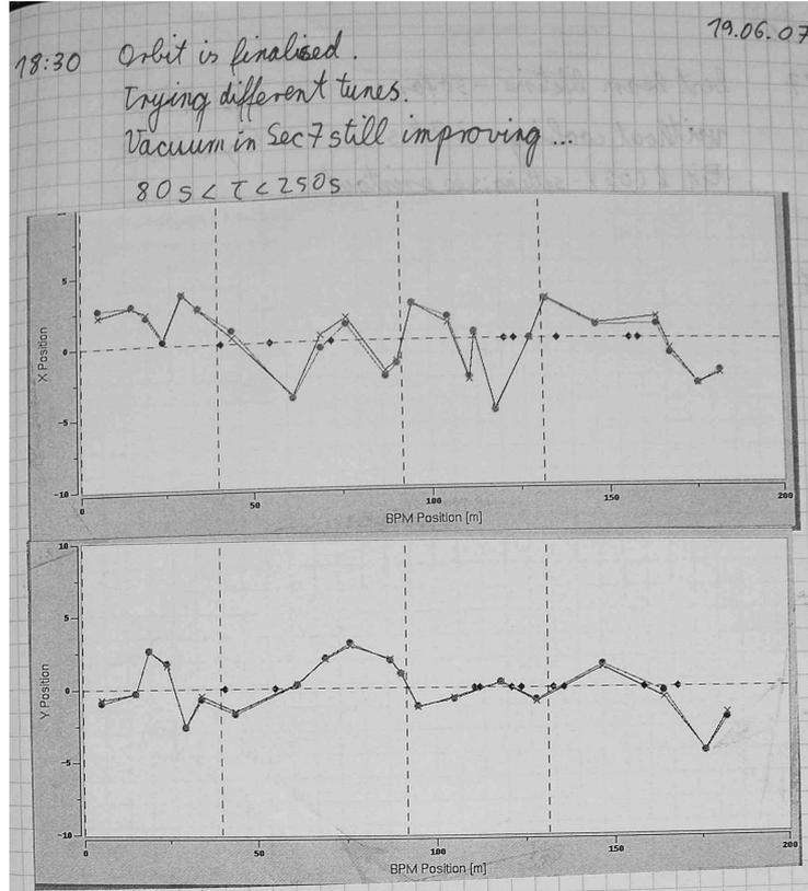
Figure 14: Beam orbit after closed orbit manipulations with all electron-cooler magnets switched off.
