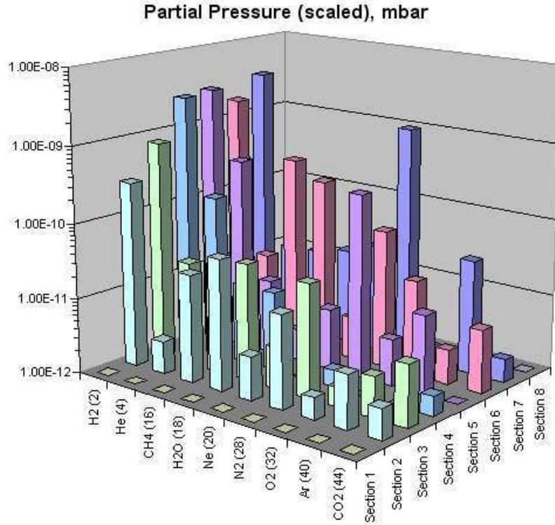
Figure 10: Main residual gas components in all COSY section at the beginning of the beam development.
