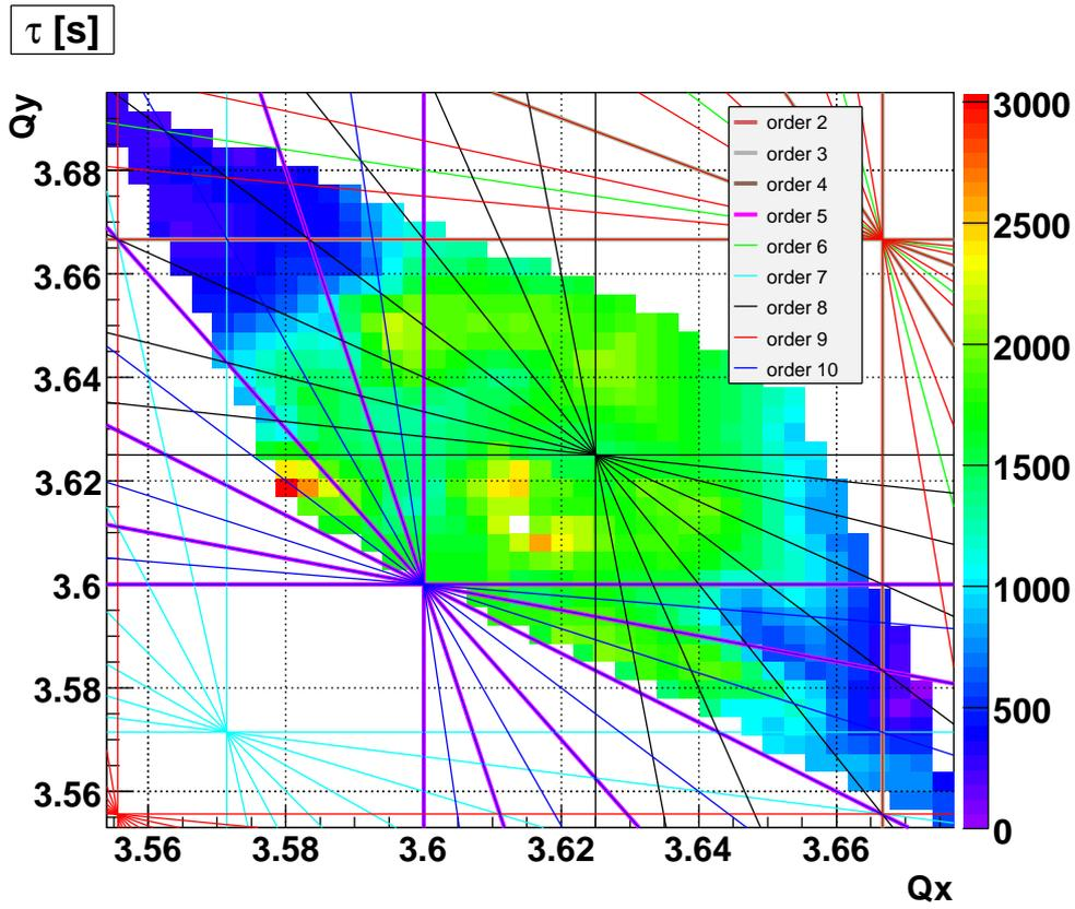
Figure 23: Lifetime as a function of the tune.
