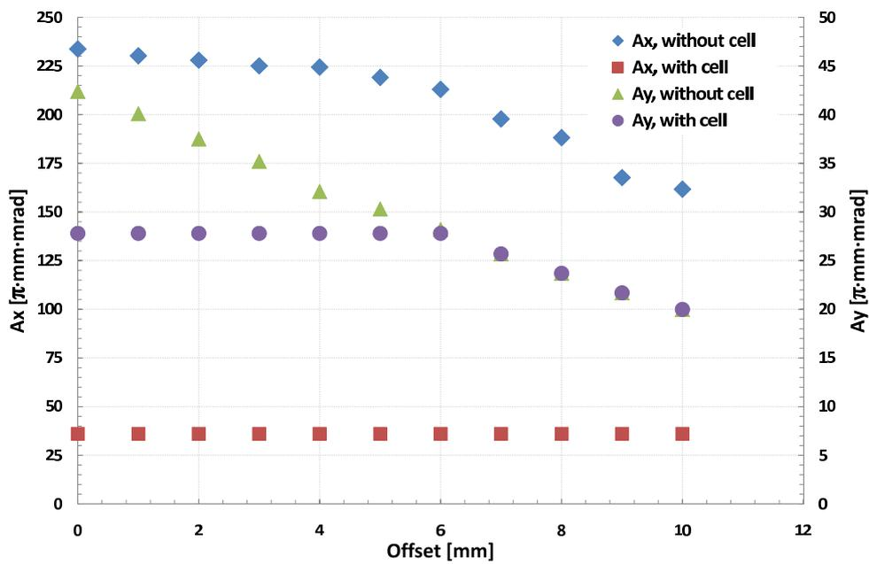
Figure 18: The plot shows the orbit deviations *versus* the vertical and horizontal acceptance with and without the storage cell.
