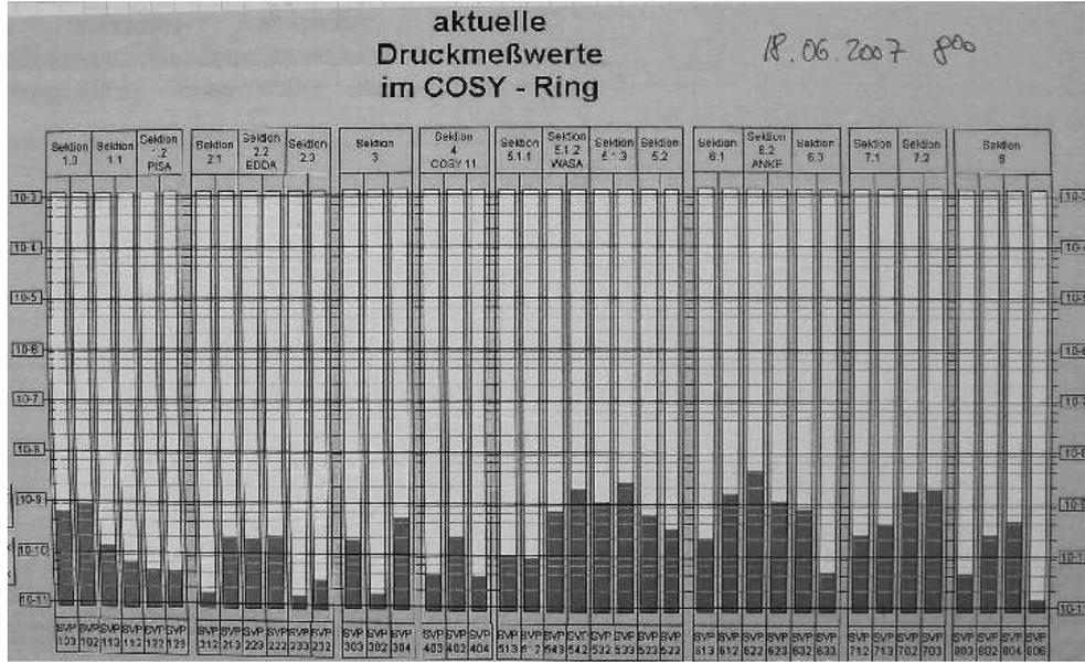
Figure 9: Pressure distribution of the COSY ring on 18th of June 2007.
