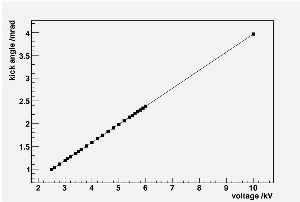
Figure 16: Calibration curve for the horizontal kicker. Voltage at the kicker *versus* kick angle  $\Theta$ . The markers show the points used for the acceptance measurement.
