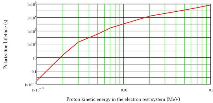
Figure 3: Polarization lifetime calculated using the spin–exchange cross section from ref. [6] as function of the proton kinetic energy in the electron rest system.
