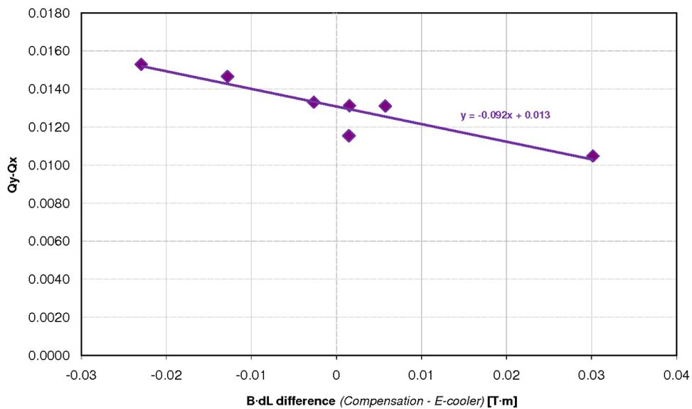
Figure 25: Tune difference as a function of the magnetic field in electron-cooler.
