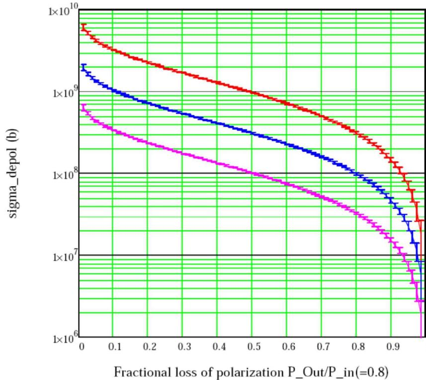
Figure 7: Estimate for the measurement of the depolarizing effect of the co-moving electrons of the cooler versus the fractional loss of beam polarization. The three curves are for kinetic energies of the proton in the electron rest frame of 0.001 (red curve), 0.01 (blue), and 0.1 (magenta) MeV. Each point reflects a 2 h measurement.
