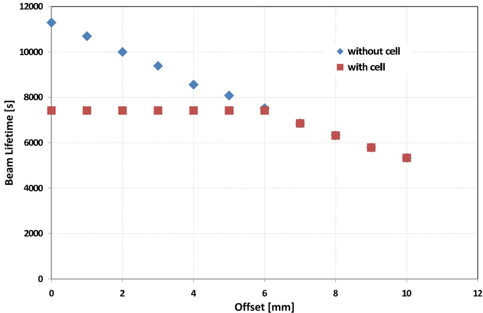
Figure 19: Beam lifetime as a function of orbit deviations.
