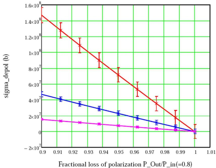
Figure 8: Estimate for the measurement of the depolarizing effect of the co-moving electrons. The color code is the same as for Fig. 7.
