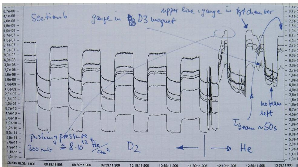
Figure 28: Pressure in section 6 with and without a deuterium and helium target.
