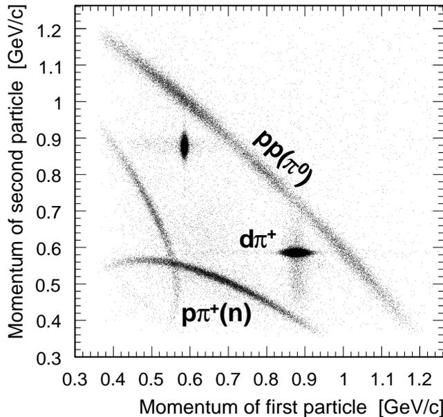
Figure 7: Scatter plot of the magnitudes of the momenta of two charged particles in the FD produced by proton-proton collisions at 800 MeV.
