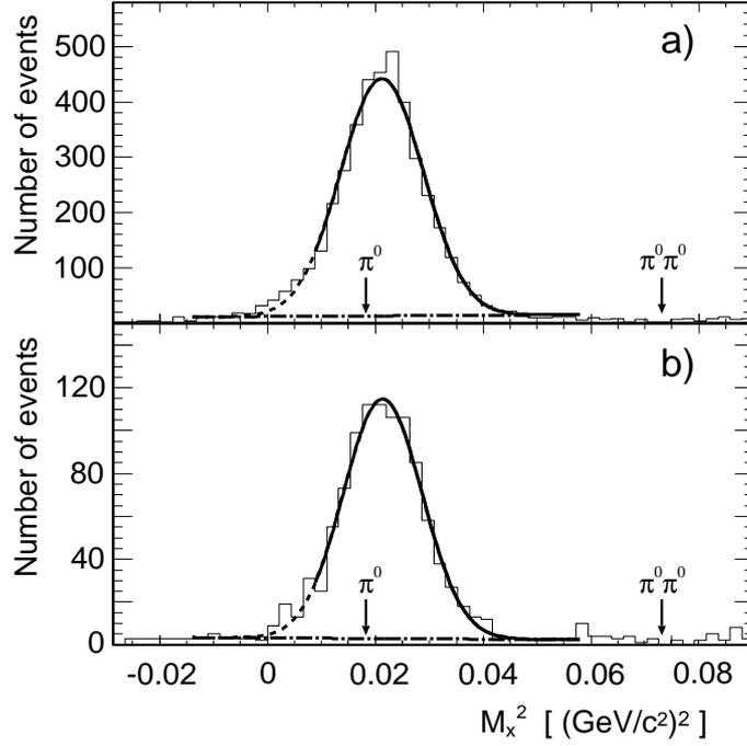
Figure 8: Distributions in the square of the missing mass for candidates for the  $pp \rightarrow ppX$  reaction with excitation energy  $E_{pp} < 3 \text{ MeV}$  when protons (a) hit different counters, and (b) the same counter. The reaction yield, obtained from fitting the data with a sum of Gaussian distribution and a constant background, is 4425 and 1008  $\pi^0$  events for cases (a) and (b), respectively.
