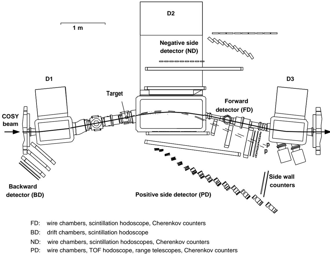
Figure 4: Schematic diagram of the ANKE experimental set-up.
