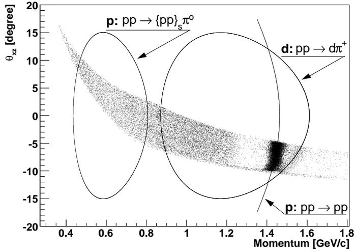
Figure 5: Experimental acceptance of the ANKE Forward Detector at the proton beam energy  $T_p=800$  MeV in horizontal angle *versus* momentum. The curves show kinematical loci for protons and deuterons from the  $pp \rightarrow \{pp\}_s \pi^0$ ,  $pp \rightarrow pp$  and  $pp \rightarrow d\pi^+$  reactions. Here,  $\{pp\}_s$  denotes a forward proton pair with zero excitation energy.
