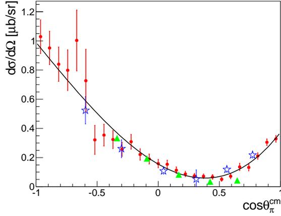
**Figure 6:** Unpolarized differential cross section for the  $pn \rightarrow \{pp\}_s \pi^-$  reaction at  $\approx 353$  MeV. The ANKE data are shown by red circles and the TRIUMF results [7] by green triangles. The arbitrarily scaled TRIUMF cross sections extracted from  $\pi^- {}^3\text{He} \rightarrow pnp_{sp}$  data [8] are also included (blue stars). The curve is a cubic fit to the ANKE data.
