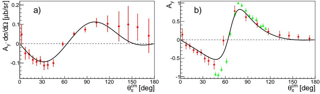
**Figure 7:** (a) The product of the measured analyzing power and differential cross section for the  $pn \rightarrow \{pp\}_s \pi^-$  reaction at 353 MeV. The curve represents the best fit of Eq. (3.4) with  $b_1$ ,  $b_2$ , and  $b_3$  terms. (b) Measured values of  $A_y$  for the  $pn \rightarrow \{pp\}_s \pi^-$  reaction showing both the ANKE (circles) and TRIUMF data [9] (triangles). The line represent the quotient of the fit in panel-a and that to the cross section.
