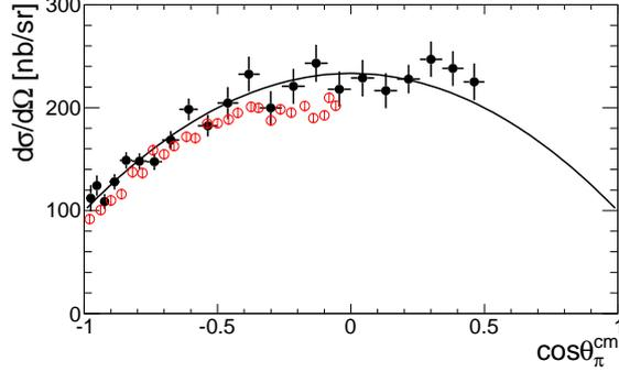
**Figure 3:** Differential cross section for the  $pp \rightarrow \{pp\}_s \pi^0$  reaction at 353 MeV as a function of the cosine of the pion c.m. angle. The solid (black) circles represent the ANKE measurements. Open (red) circles are CELSIUS data obtained at 360 MeV [6]. The curve is a linear fit in  $\cos^2 \theta_\pi$  to our data.
