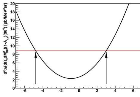
**Figure 3.** Dependence of  $(1 - A_{x,x})d\sigma/d\Omega$  at  $90^\circ$  on the  $d$  LEC. The value  $d = 3$  favoured by the theory is shown by an arrow. The horizontal line corresponds to the measured value at  $d = 3$ , while another arrow at  $d \sim -5$  points to the second solution for this measured value.
