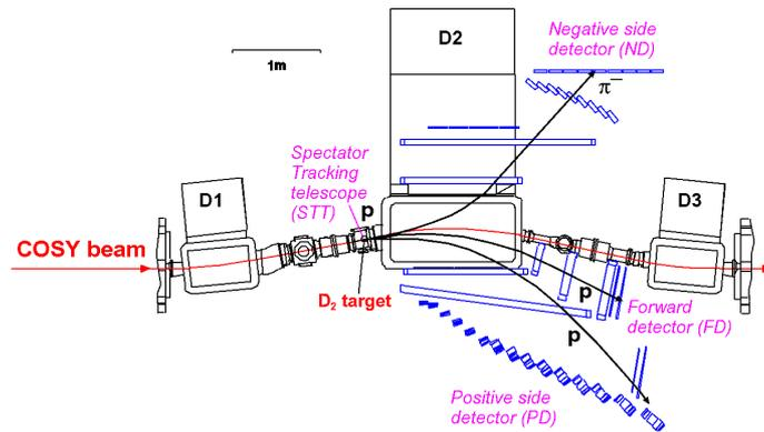
**Figure 1.** Top view of the ANKE setup at COSY. The positions of the dipole magnets D1, D2, D3, the cluster target spot, the Forward (FD), Positive (PD), Negative (ND) detector systems and the Silicon Tracking Telescope (STT), are shown.
