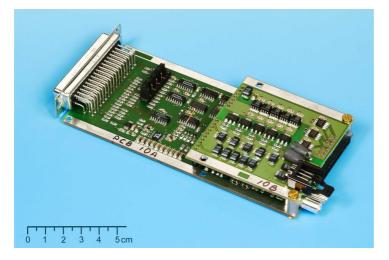
opto-decoupling from the detector bias and analog and digital chip control
