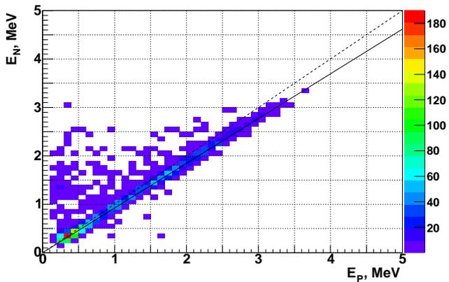
**Fig. 1:** Typical  $E_N$ – $E_P$  correlation plot for a segment from  $P$ -side of the thin plane with respect to all  $N$ -segments connected to a reference chip. Dash line corresponds to  $E_N = E_P$ , solid line — fit result.
