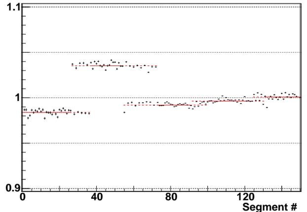
**Fig. 2:** The typical correction factors for the  $300\ \mu\text{m}$  thick layer: segment-wise (black) and chip-wise (red).
