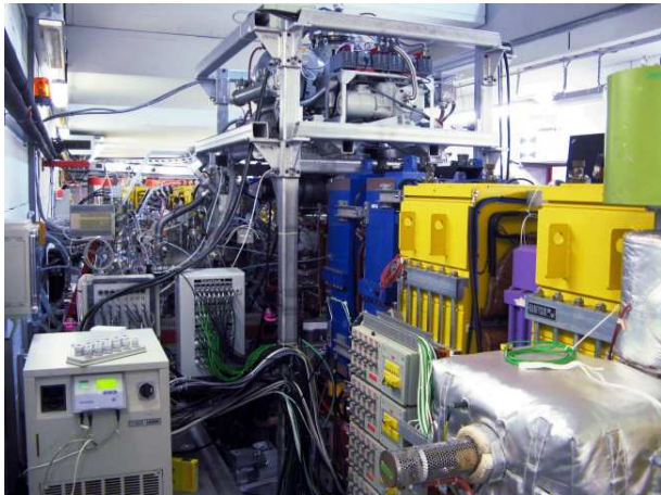
Fig. 22: The PAX installation at COSY showing the newly installed quadrupoles (blue color and the support structure for the polarized source, the polarimeter and the target chamber.
