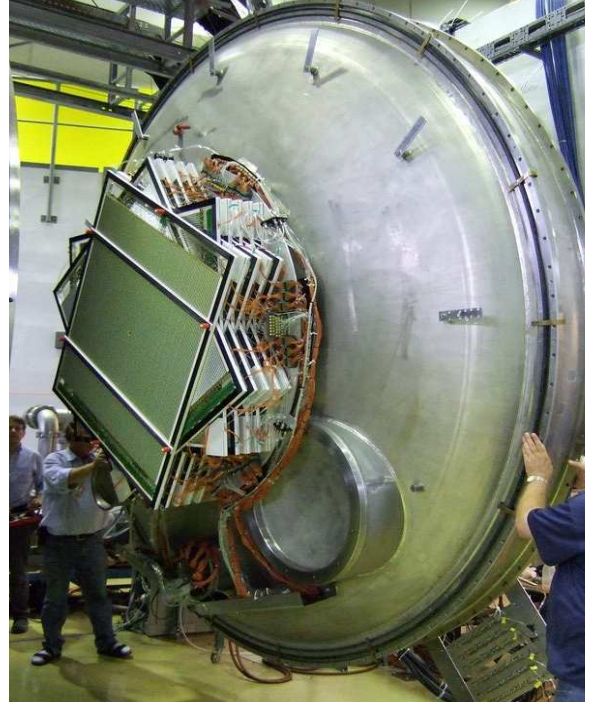
Fig. 13: The Straw Tube Tracker at the COSY-TOF front-cap before its final mounting to the TOF vacuum barrel (at left side). The tracker consists of a stack of 15 straw double-layers.
