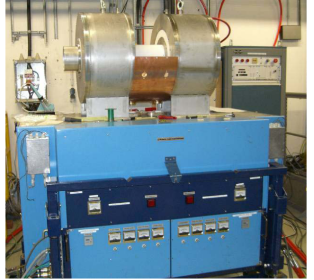
Fig. 45: Accelerating cavity for HESR installed on top of the former COSY tube amplifier.
