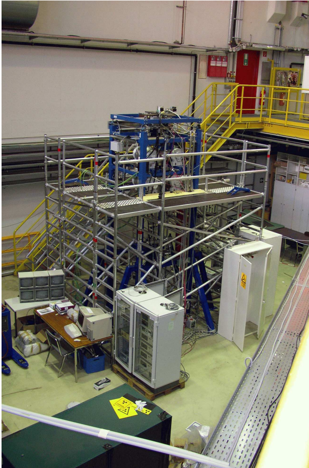
Fig. 9: Test setup of the WASA pellet target at COSY with pellet generator (top), a dummy vacuum chamber around the nominal interaction zone, and pellet beam dump (bottom).
