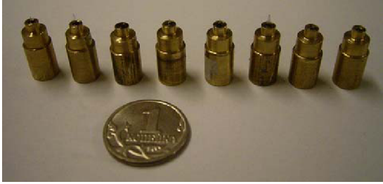
Fig. 57: Nozzles from quartz glass and brass for droplet production.
