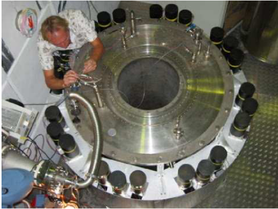
Fig. 26: ATRAP-II magnet and C. Storry during assembly.
