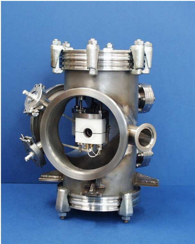
Fig. 1: Deflector chamber (height about 40 cm) with the spherical deflector and the two lenses (visible is one of the lenses within the teflon insulation with the deflector behind it).
